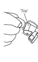
Once connector is fully inserted into the Tallon Socket, ensure the wide tab of the locking cam is on the left and the word 'Top' is visible on the top of the cam.
